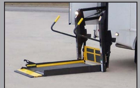
Optional ADA wheelchair lift mounted in the rear or the bus
